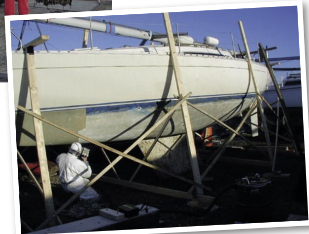
The osmosis-riddled gel coat is peeled back
