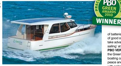
PERFORMANCE: With 165hp of diesel grunt you should get a top speed of 15 knots, but the super-displacement hull is most economic on fuel at around 7 knots, where it gets around 5 miles per gallon. The 7kW electric engine will produce 4 knots for around five hours from a fully charged 120Ah battery array. The 1.3kW solar panel 'power plant' will recharge a flat set
