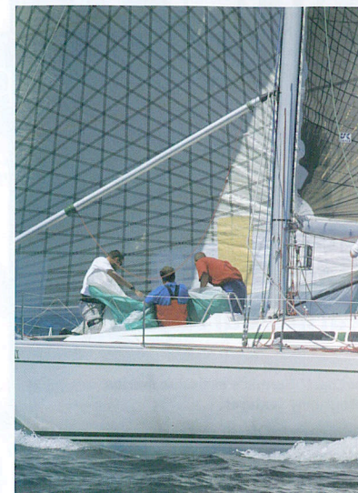
▲ Laminated sails are more efficient than woven sails
