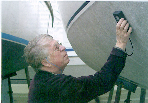
Checking for moisture content in the hull, which can lead to blistering
