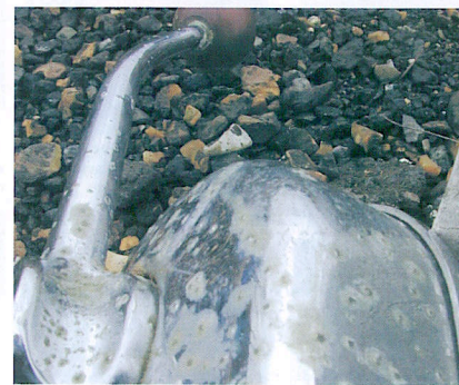
▲ This chromium-plated engine control looked like this after only a few months of being left with salty moisture on the surface
