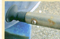
▲ Stainless steel needs to be well polished to avoid rust bleeding.
