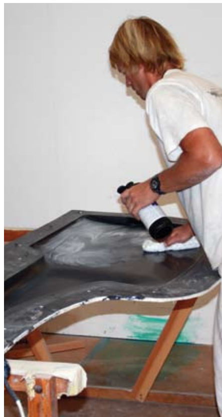
A mould is made from the rudder's plug and polished ready for the first blade to be laid up
