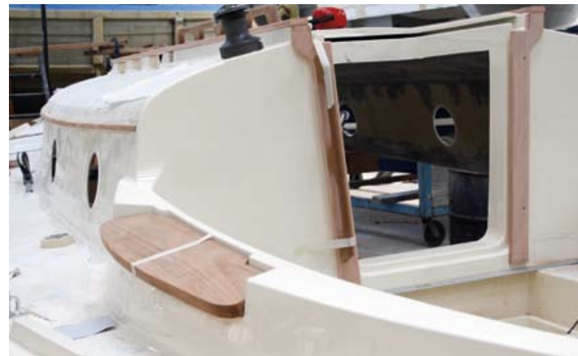
Hardware and timber trim are fitted to the deck and cockpit
