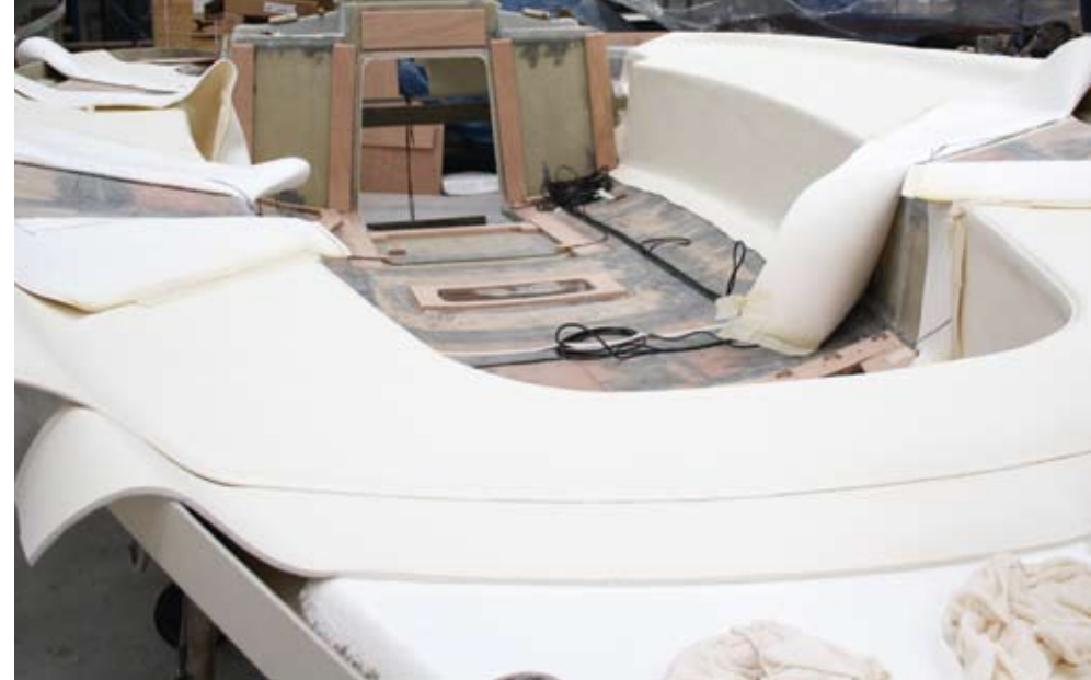
Now it's time to fit the vinyl, which is stuck to the underside of the decks and the coachroof sides
