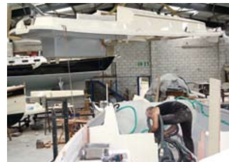
Everything that can be fitted to the hull and deck while they're still separate has been fitted. Now it's time to join the two together - they're screwed and bonded - and finish the boat
