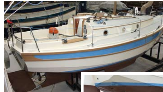
The final chance to drop the centreplate to make sure all's well before she finally hits the water. Note the balance on the leading edge of the rudder and the blades of the three-bladed prop in their feathered position
