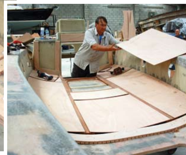
Then the plywood panels themselves are dropped in for a test fit
