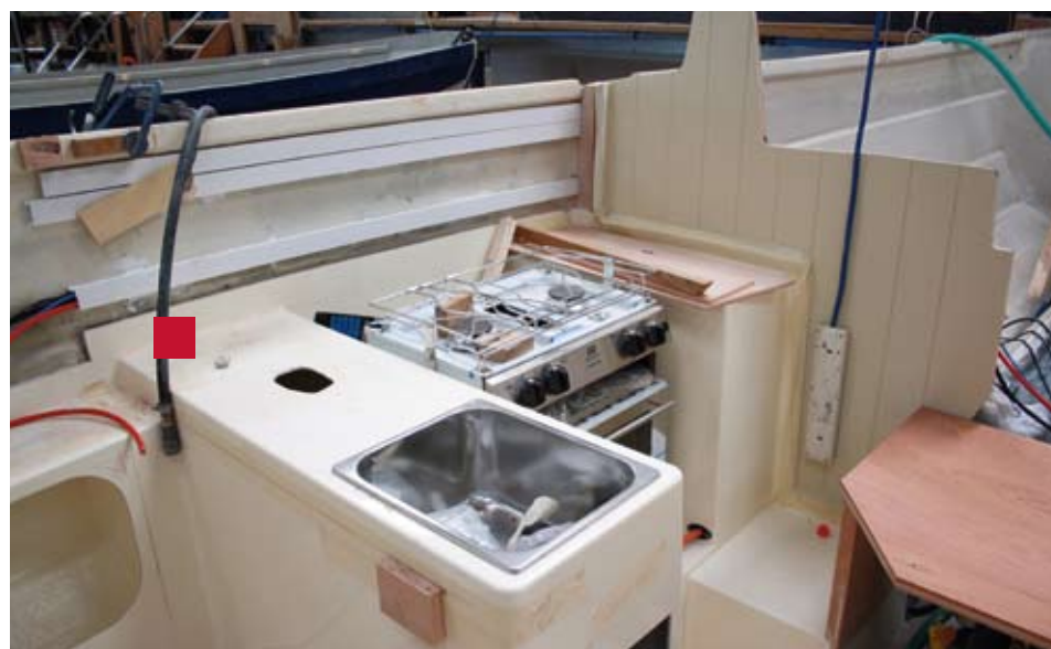
In go the sink and cooker. The coolbox will be outboard of the sink. Note the tongue-and-groove effect on the bulkhead, which is achieved by use of a router
