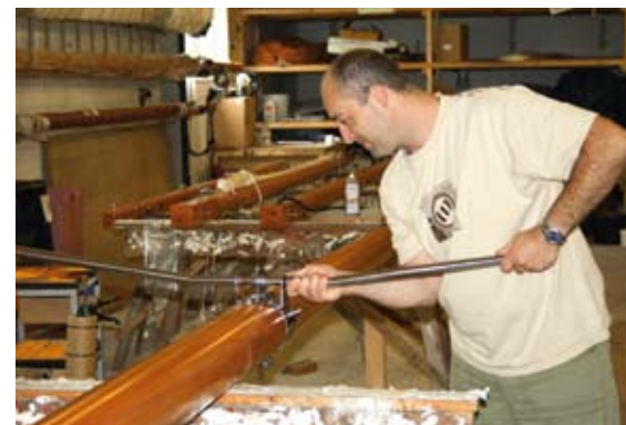
The spars have arrived from manufacturers Collars and are being dressed in the rigging shop. The spreaders are angled slightly, but most of their sweep-back is achieved by their being set abaft the mast
