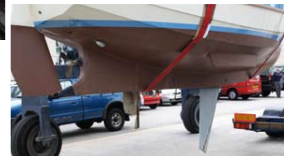
The final chance to drop the centreplate to make sure all's well before she finally hits the water. Note the balance on the leading edge of the rudder and the blades of the three-bladed prop in their feathered position
