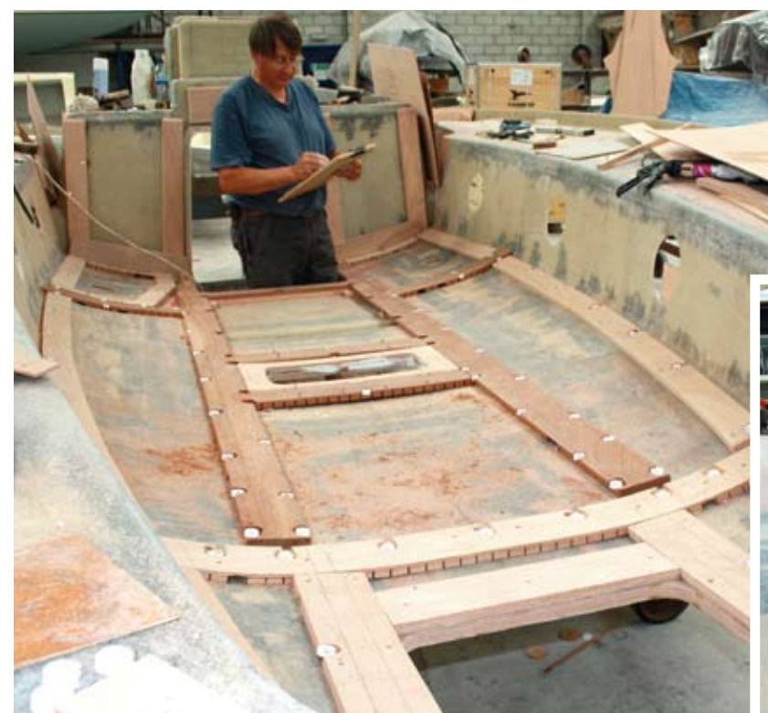
With the decision taken to use vinyl rather than a glassfibre moulding for the headlining, the framework for the plywood panels is fitted to the underside of the deckhead
