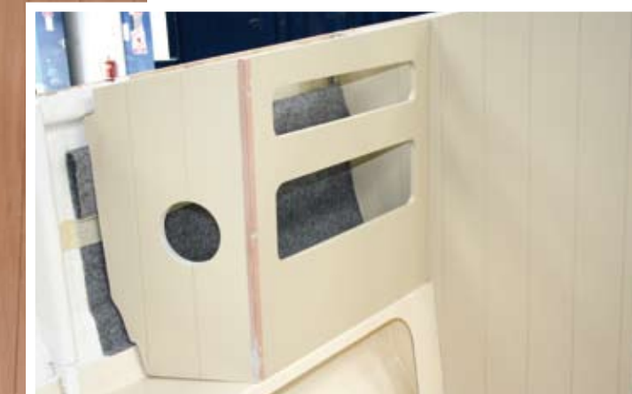
...and this is how it looks when shaped, trimmed, routed, painted and lined inside with carpet. It doubles as a knee in way of the chainplates to reinforce the topsides
