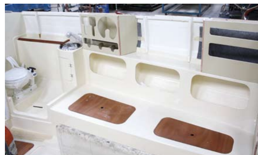
With the joinery units fitted and hull sides flow-coated, it begins to look more like a boat's interior. The space beneath the saloon berths on both sides is used for stowage
