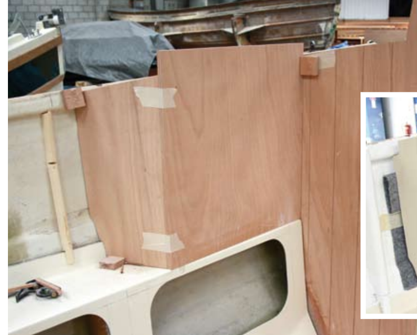
This is how the locker to port abaft the main bulkhead starts out...
