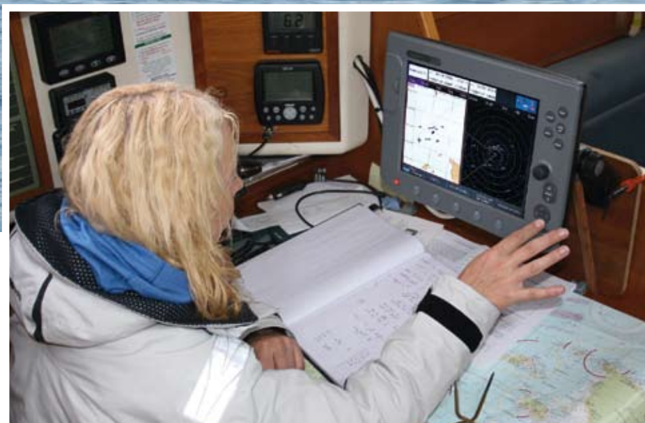
We navigated with Navionics electronic charts, and plotted our position on the paper chart every hour
