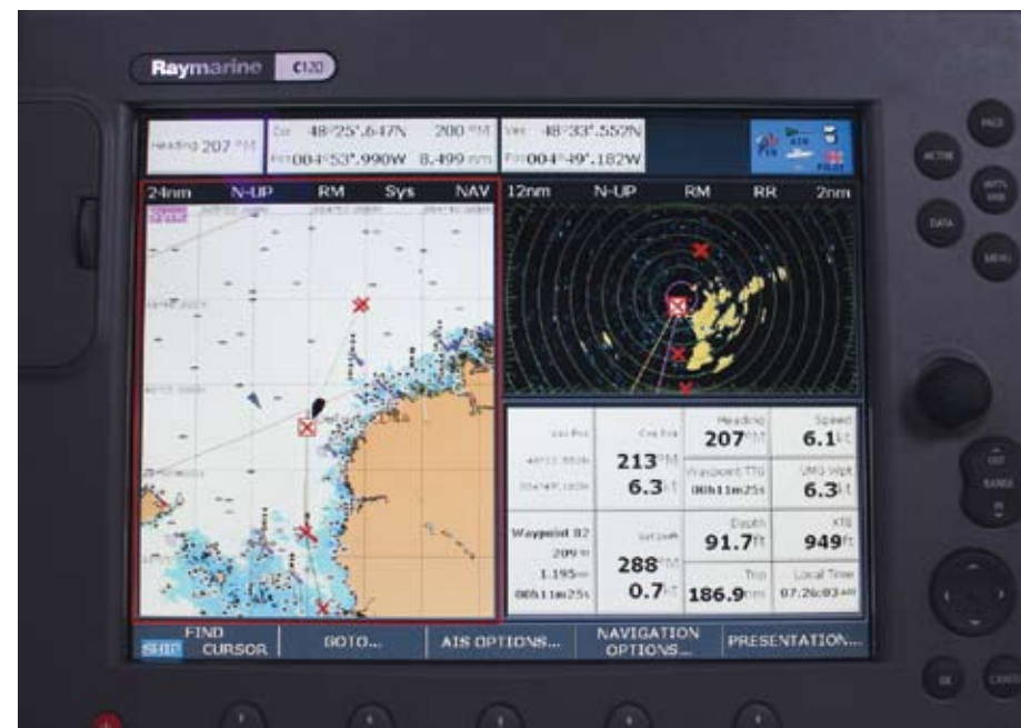
The ability to show your position and waypoints on both chart and radar displays made the Chenal du Four easy. Note the AIS ship on the chart. You can also overlay chart, radar and AIS on one image
